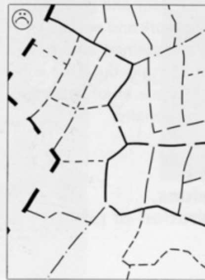
Fig. 2.47 Poorly proportioned line work (left); Well proportioned line work (right)
