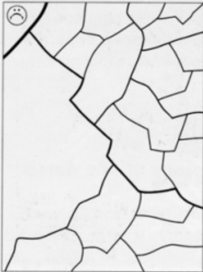
Fig. 2.46 Line width separation too small (left); Good line width separation (right)
