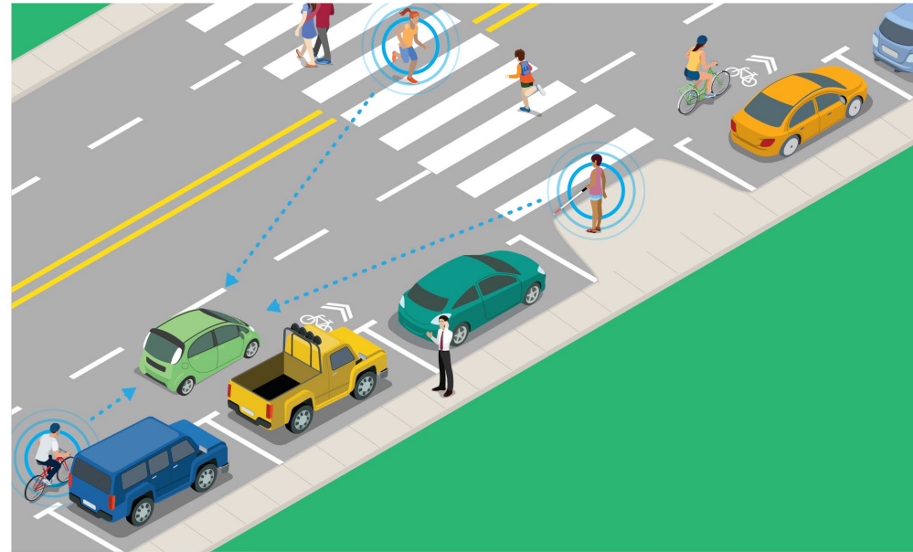
Figure 3. Vehicle to pedestrian or bicyclist technologies (V2X) could aid in detection of and communication with pedestrians and bicyclists, but an array of technology and equity issues must still be addressed.
